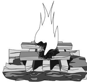
FIG. 4.7 Burning firelighter module on stack of firewood
